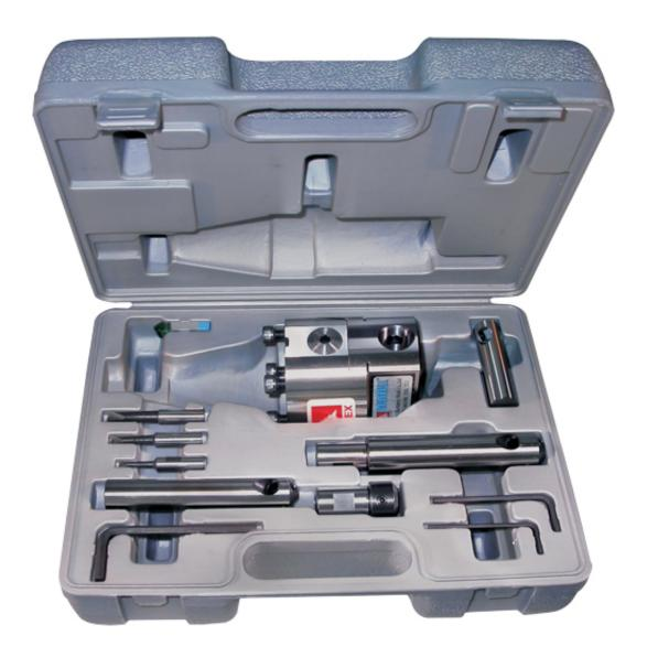
Part No Description Weight Units: per VBH Boring Head 82mm 4.60
