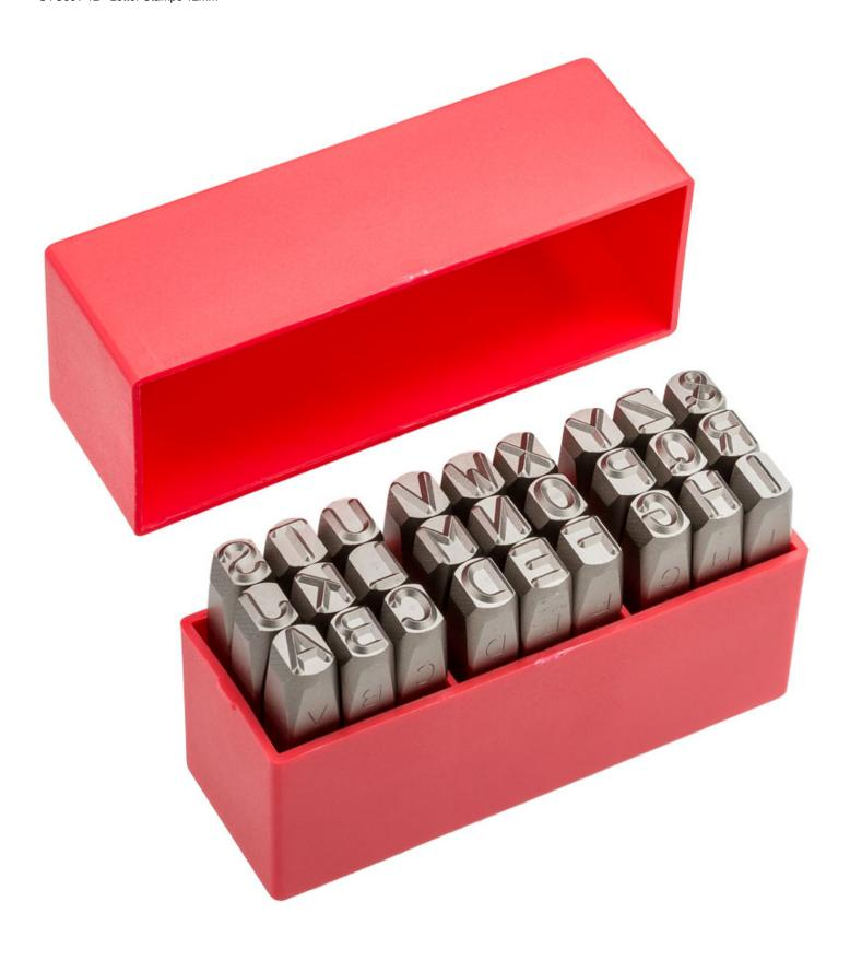
Part No Description Weight Units: per GYC601-12 Letter Stamps 12mm 4.40 Individually marked with the size on the side Tapered sides to stamp head Made from CRV (6150), sandblast finish
